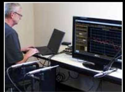
Total Cal operates in an ordinary room. No anechoic chamber is required
